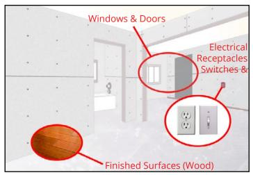
Temporarily block windows and doors; cover electrical receptacles and switches; protect finished surfaces.
