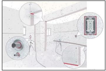
Allow the particles to build up around any gaps and holes to seal leakage areas without coating surfaces.
