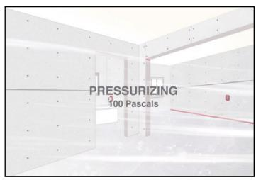
Pressurize the space and its air leakage with a computer-controlled atomization system.
